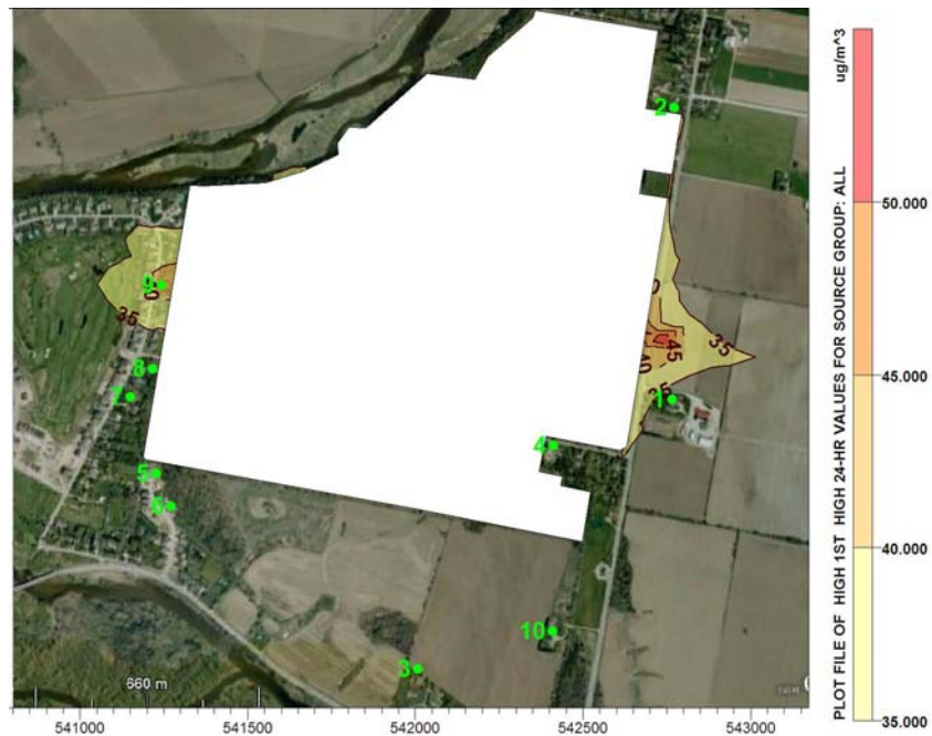
FIGURE D7-3 – HIGHEST PREDICTED 24-HOUR AVERAGE PM 10 CONCENTRATIONS - PHASE 7 – 50% SCREENING AT FACE 50% PROCESSING
