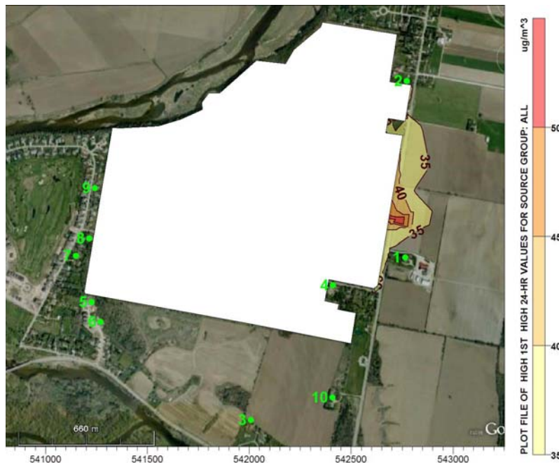
FIGURE D5-1 – HIGHEST PREDICTED 24-HOUR AVERAGE PM 10 CONCENTRATIONS -PHASE 5 – 100% SCREENING AT FACE
