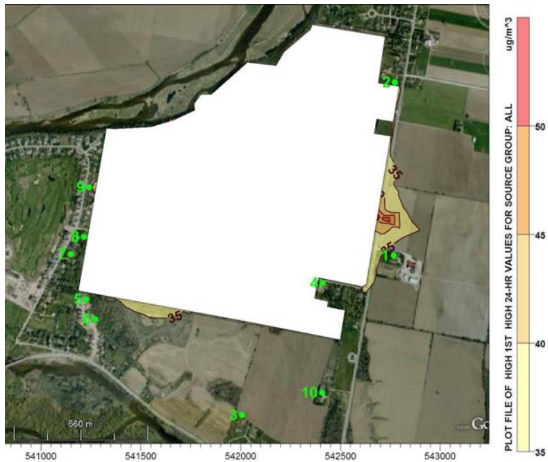
FIGURE D3-3 – HIGHEST PREDICTED 24-HOUR AVERAGE PM 10 CONCENTRATIONS - PHASE 3 – 50% SCREENING AT FACE 50% PROCESSING
